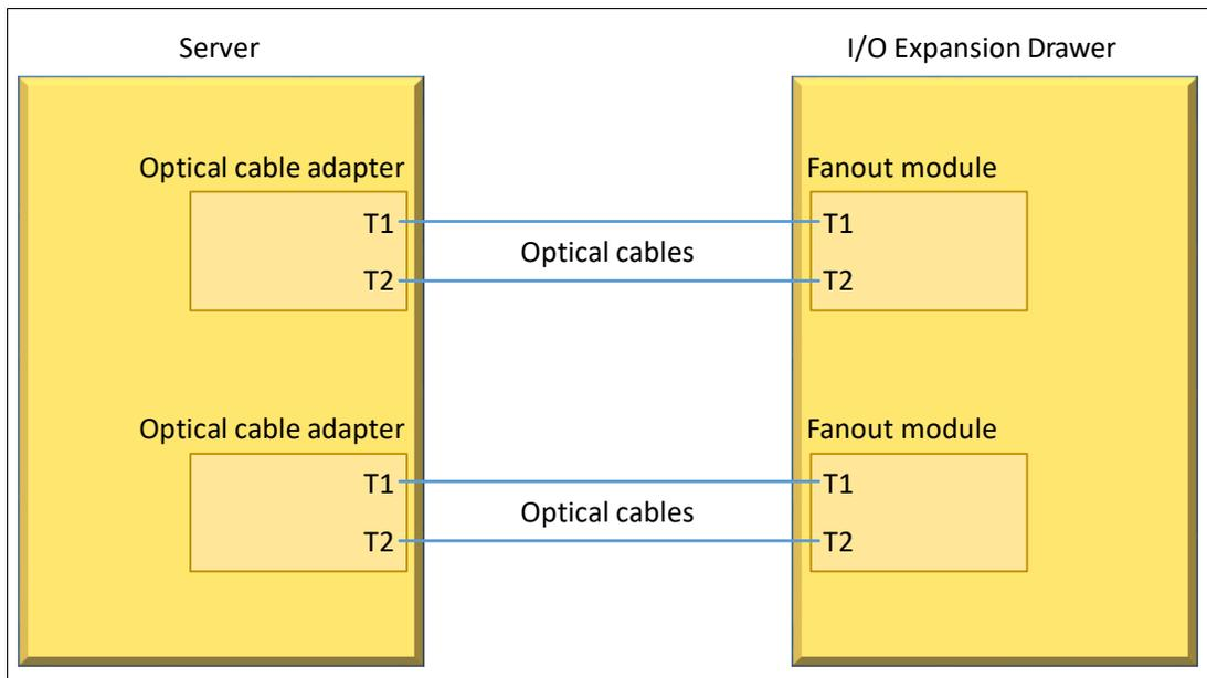
Figure 3-10 Typical optical cable connections
