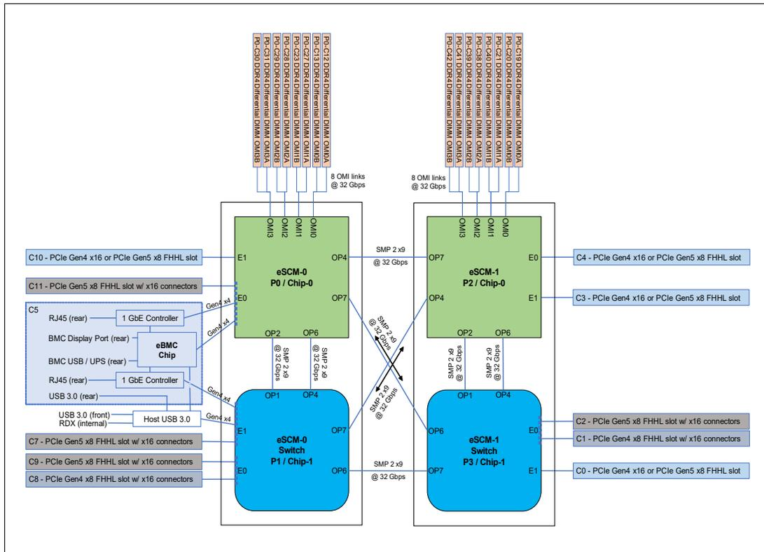
Figure 2-2 Logical diagram of the Power S1022s server in a 2-socket configuration
