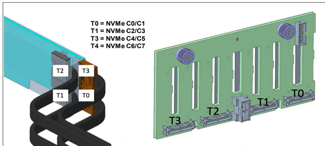
Figure 3-3 Connector locations for JBOF card and NVMe backplane
