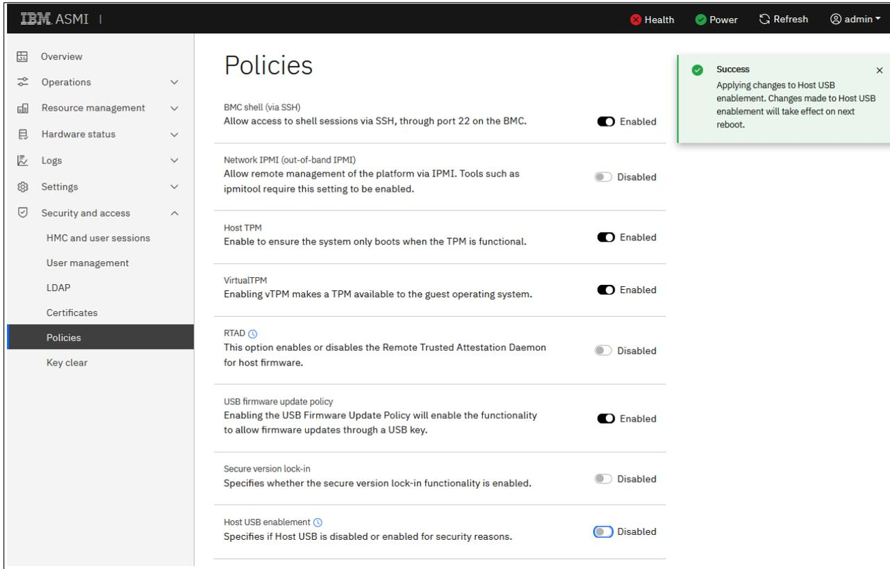
Figure 2-35 Switching off the USB ports of the server
