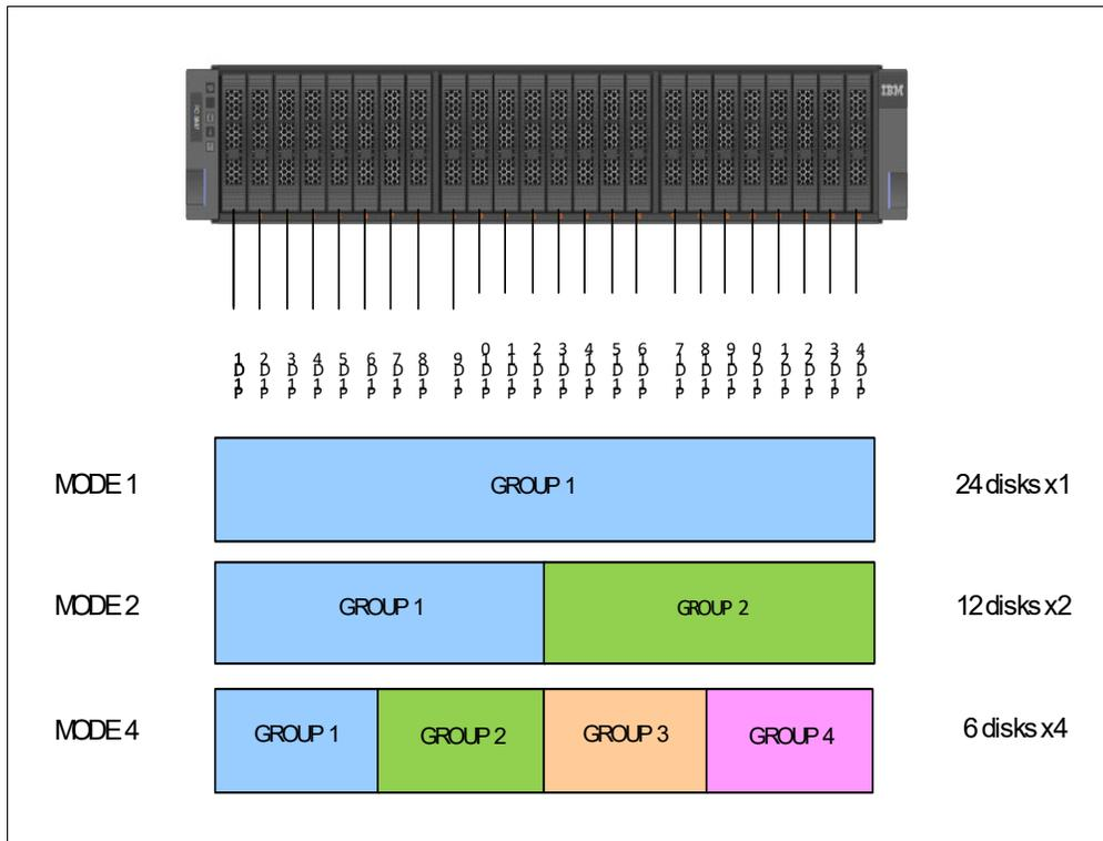
Figure 3-15 Front view of the ESLS storage enclosure with mode groups and drive locations
