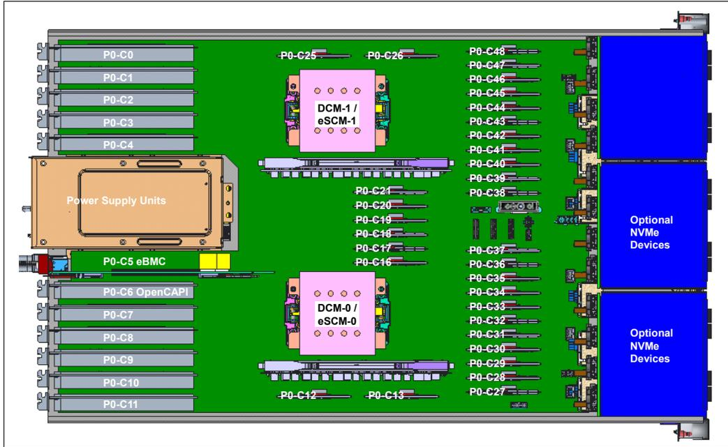
Figure 2-19 Memory module physical slot locations and DDIMM location codes
