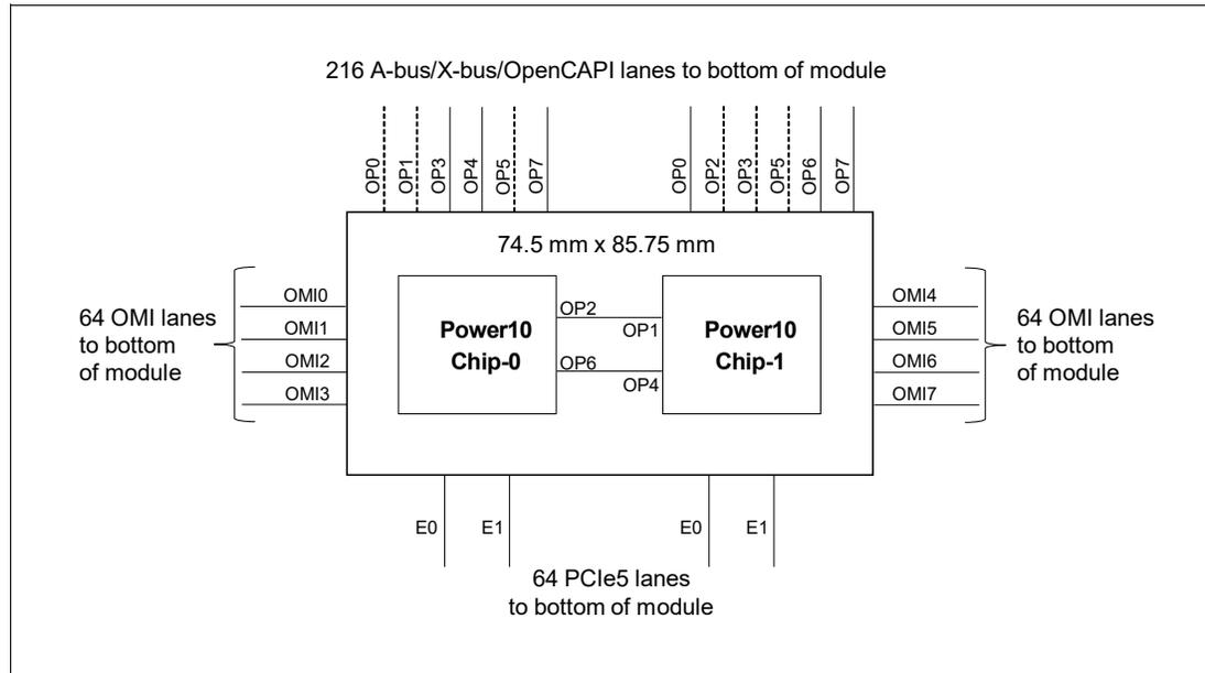
Figure 2-6 Power10 dual-chip module logical diagram
