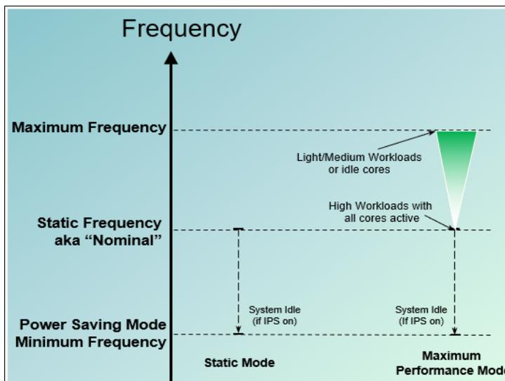
Figure 2-14 Power10 power management modes and related frequency ranges
