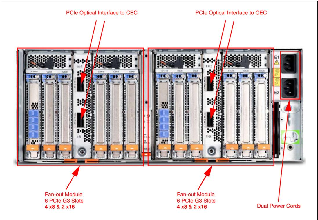
Figure 3-6 Rear view of the PCIe Gen3 I/O expansion drawer
