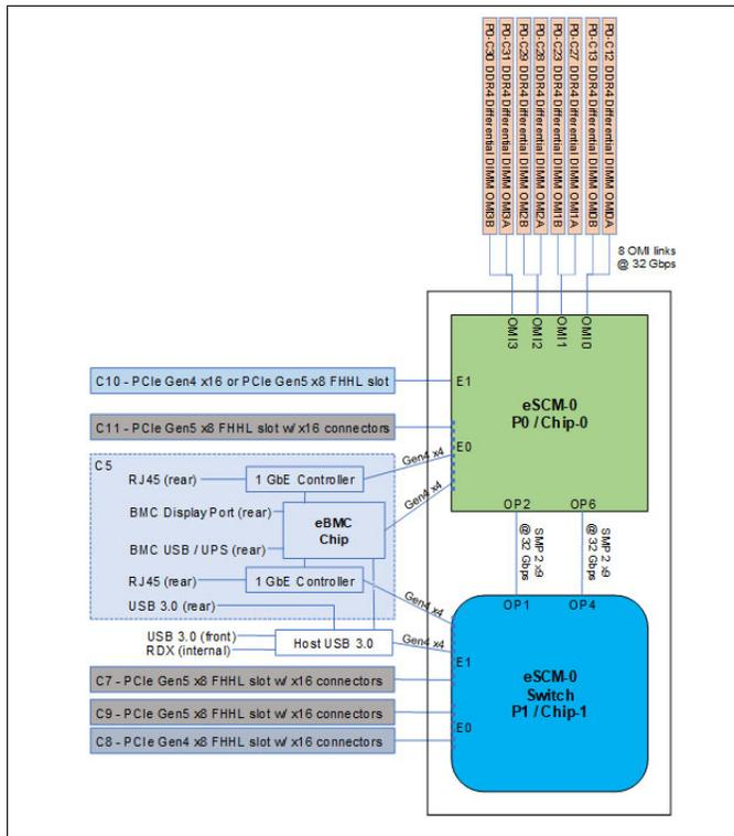
Figure 2-3 Logical diagram of the Power S1014 server with eSCM
