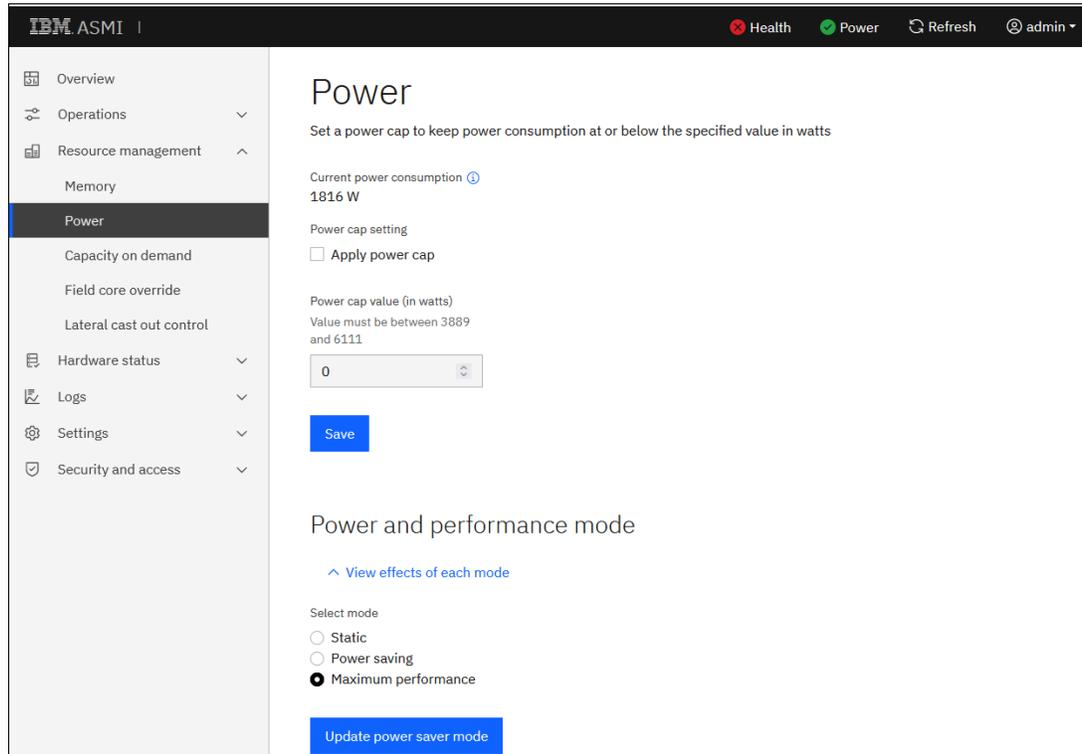
Figure 2-15 ASMI menu for Power and Performance Mode setup
