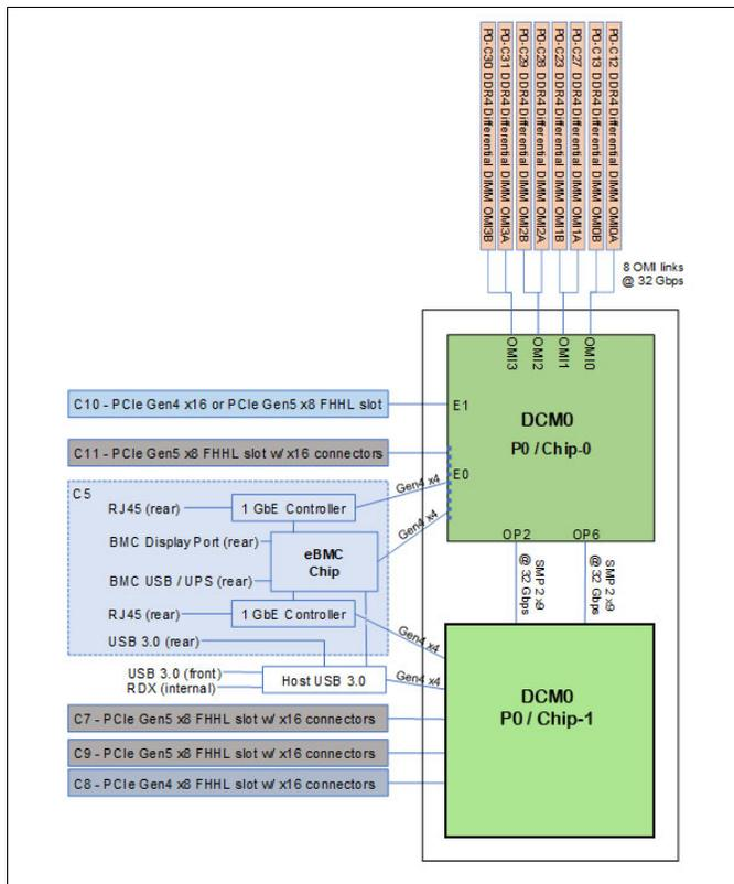
Figure 2-4 Logical diagram of the Power S1014 server with DCM
