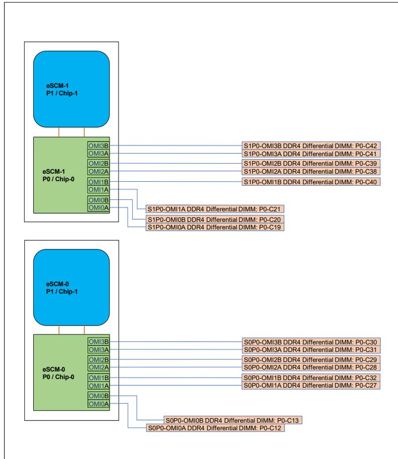
Figure 2-18 Memory logical diagram of eSCM-based Power S1022s server
