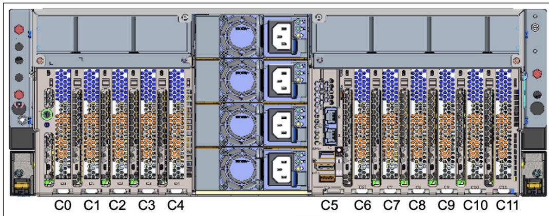
Figure 2-30 Rear view of a Power S1024 server with PCIe slots location codes
