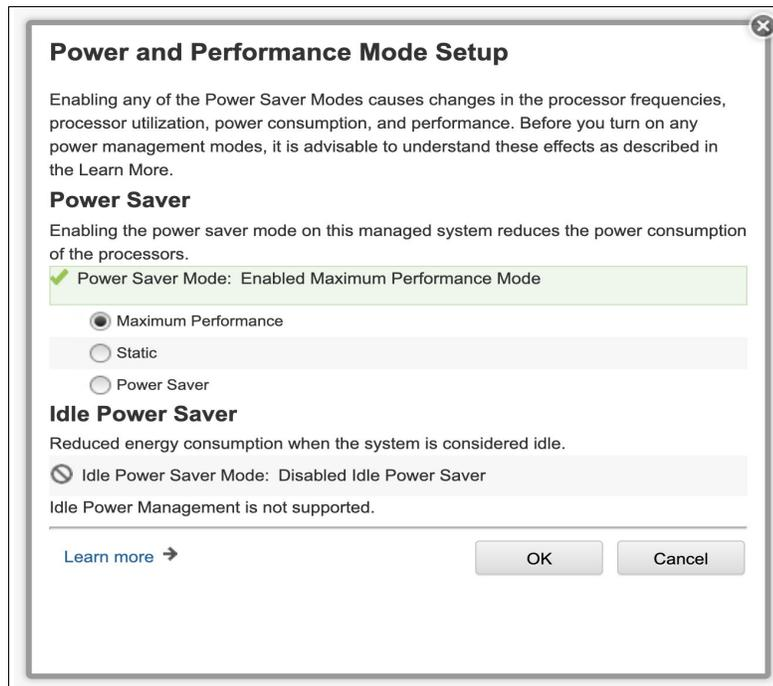
Figure 2-16 HMC menu for Power and Performance Mode setup
