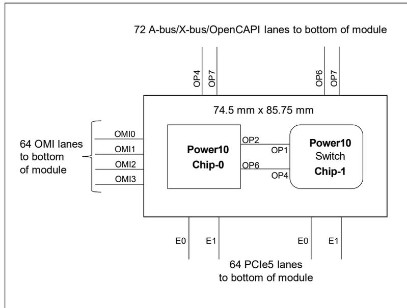
Figure 2-8 Power10 entry single chip module logical diagram
