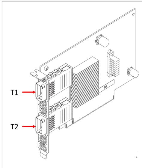
Figure 3-8 PCIe3 x16 to CXP Converter Adapter (#EJ24)
