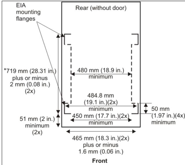
Figure 3-18 Rack specifications (top-down view)
