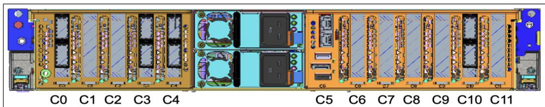
Figure 2-29 Rear view of Power S1022s and S1022 servers with PCIe slots location codes
