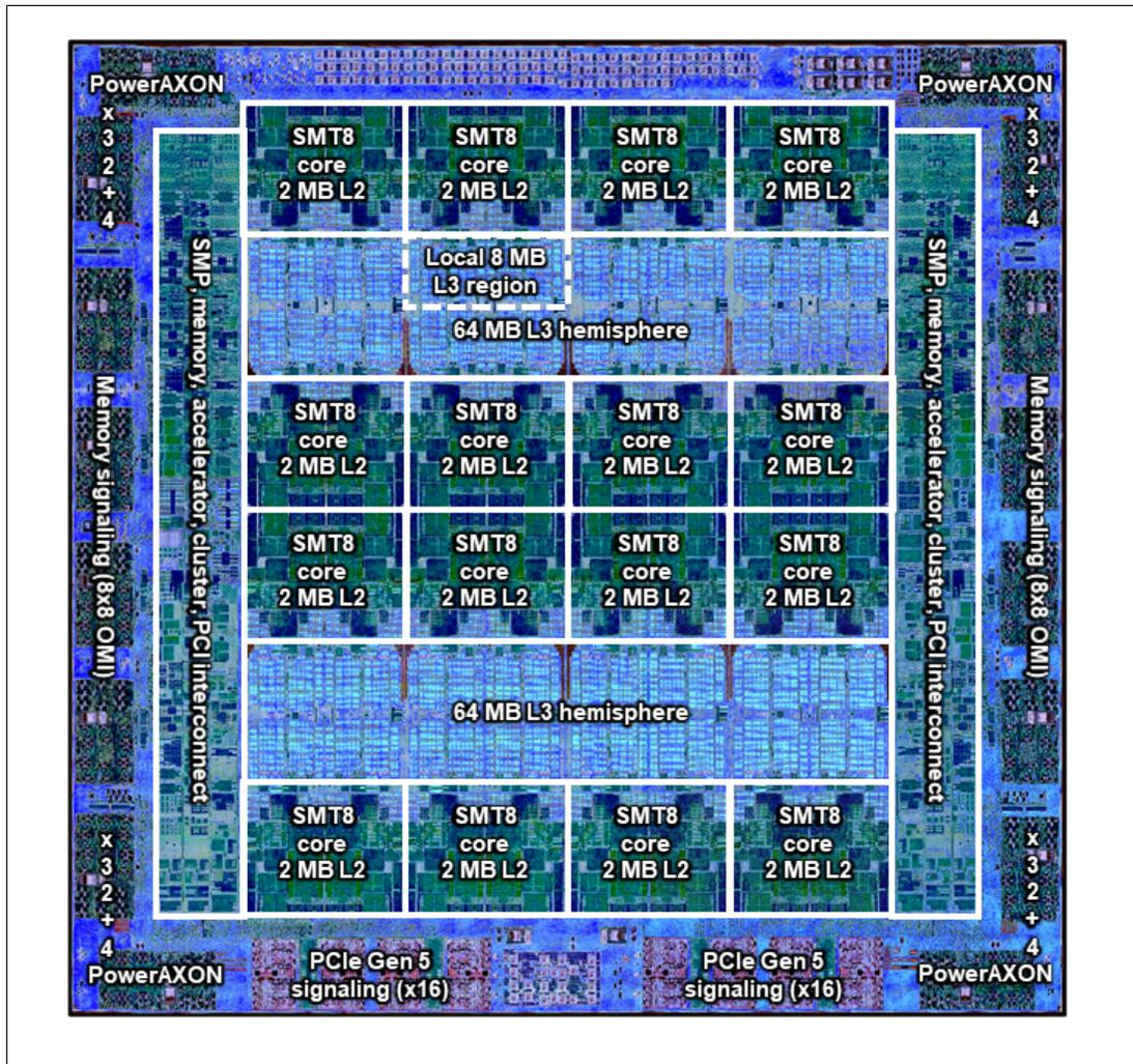
Figure 2-5 The Power10 processor chip
