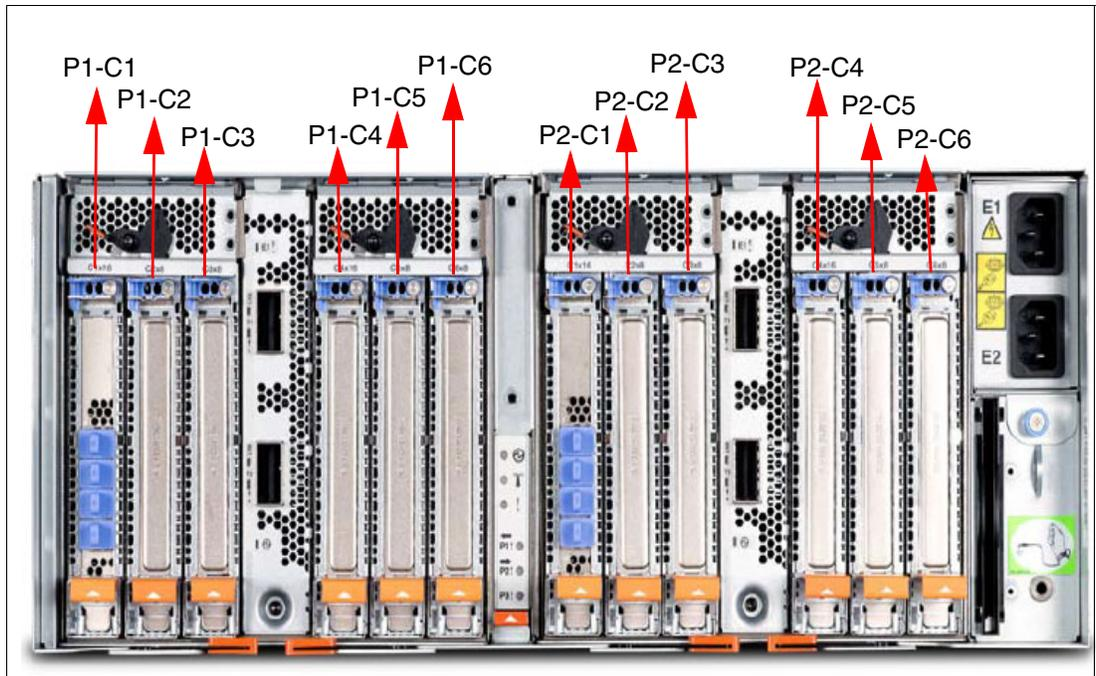
Figure 3-7 Rear view of a PCIe Gen3 I/O expansion drawer with PCIe slots location codes
