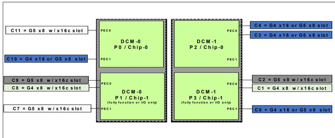
Figure 2-27 PCIe slot internal connections of a 2-socket DCM server
