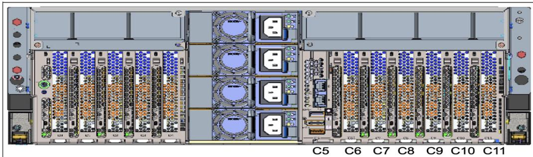
Figure 2-28 Rear view of a Power S1014 server with PCIe slots location codes
