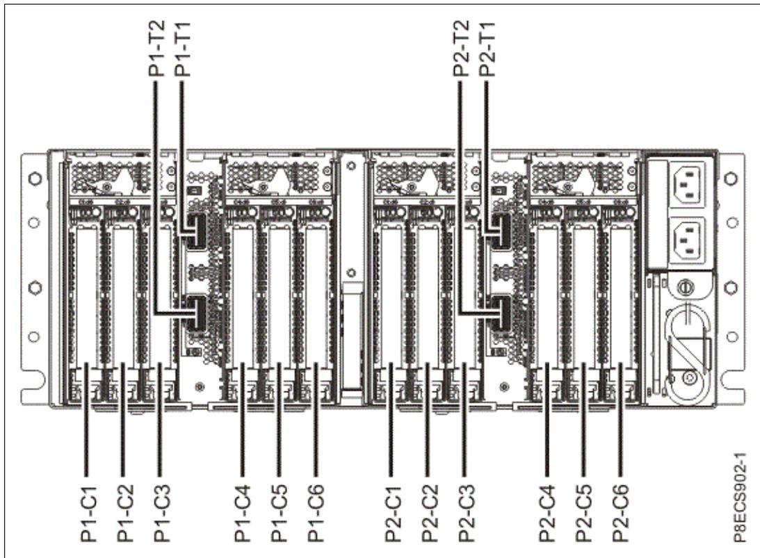
Figure 3-9 Connector locations for the PCIe Gen3 I/O expansion drawer
