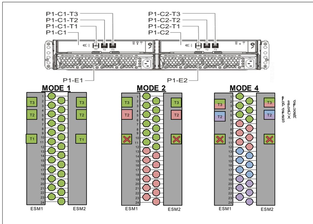
Figure 3-16 Rear view of the EXP24SX with location codes and different split modes
