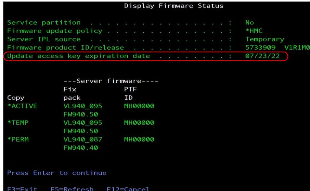
Figure 1-7 Display Firmware Status window
