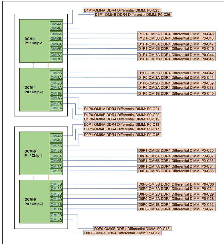
Figure 2-17 Memory logical diagram of DCM-based Power S1022 and Power S1024 servers
