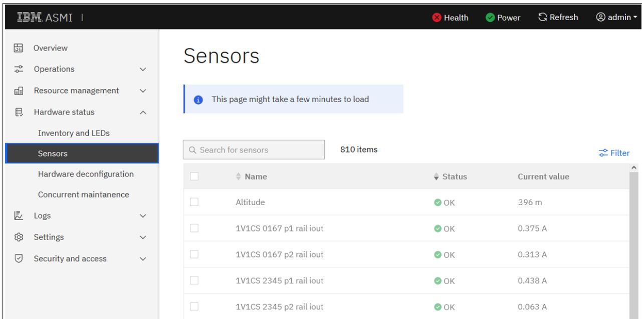
Figure 2-33 ASMI sensors
