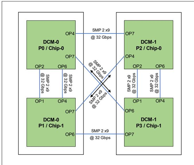
Figure 2-12 SMP connectivity for Power S1022 or Power S1024 servers in 2-socket configurations
