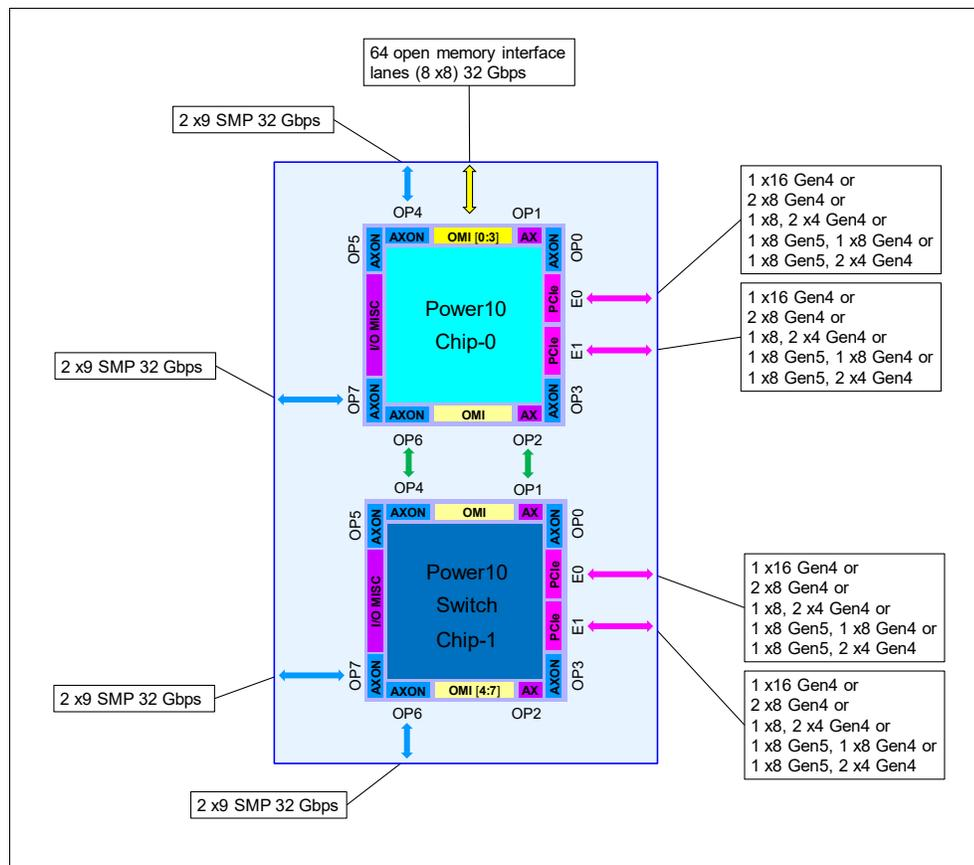
Figure 2-9 Power10 entry single chip module physical diagram
