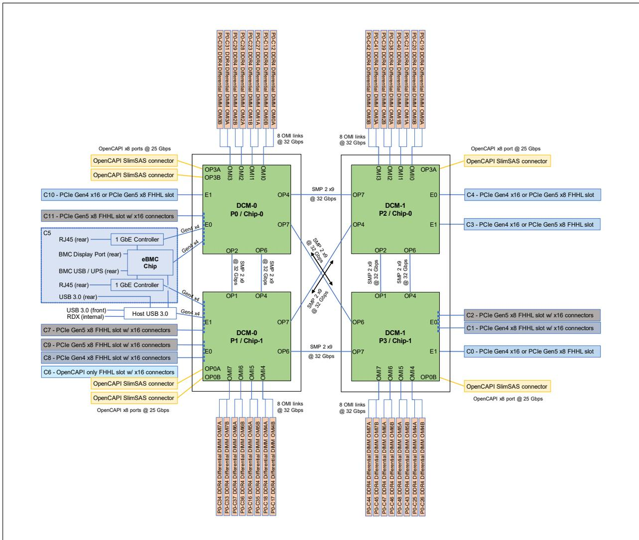
Figure 2-1 Logical diagram of Power S1022 or Power S1024 servers in 2-socket configurations
