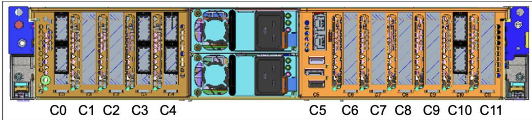
Figure 1-6 PCIe adapter slot locations on the Power S1022s and S1022 server models
