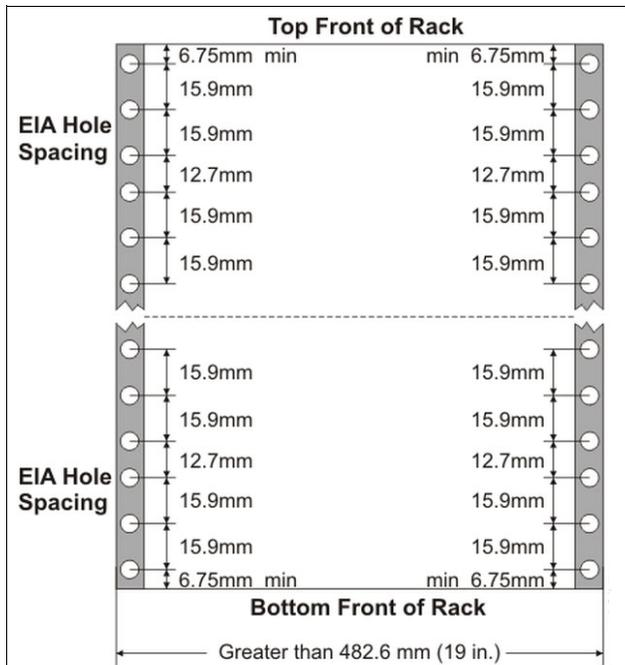
Figure 3-19 Vertical distances between mounting holes
