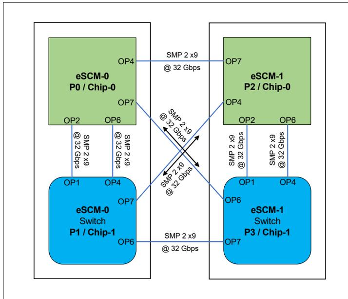
Figure 2-13 SMP connectivity for a Power S1022s server in 2-socket configuration
