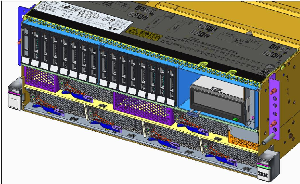
Figure 3-4 The Power S1014 and S1024 servers with two storage backplanes and RDX drive
