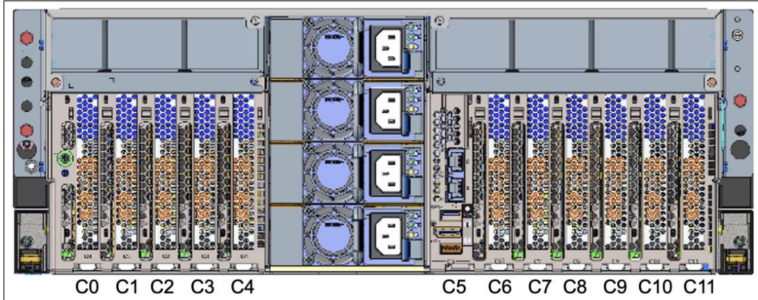
Figure 1-5 PCIe adapter slot locations on the Power S1014 and S1024 server models
