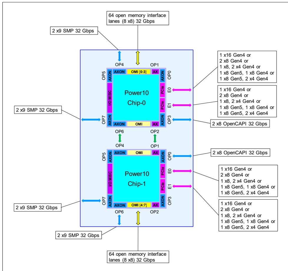
Figure 2-7 Power10 dual-chip module physical diagram
