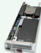
SBA-4119SG GPU Model with 2 GPUs, M.2 NVMe
