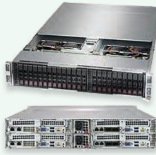
AS -2124BT-HTR 2U System with 4 hot-pluggable Dual-Processor Server Nodes with U.2 SATA
