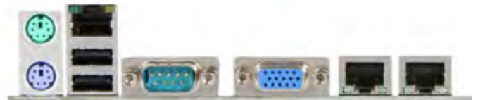
■ FIG 6: THE DEDICATED IPMI LAN IS ABOVE THE USB PORTS ON THIS SUPERMICRO X8STI-F MOTHERBOARD
