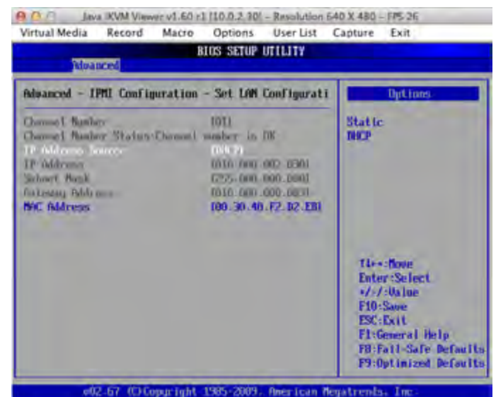
■ FIG 10: IPMI CONFIGURATION IN THE MOTHERBOARD BIOS USING KVM/IP FROM MAC OS X
