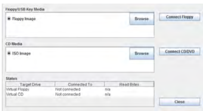
■ FIG 5: EXAMPLE MEDIA REDIRECTION FUNCTION OF SUPERMICRO'S KVM OVER IP INTERFACE
