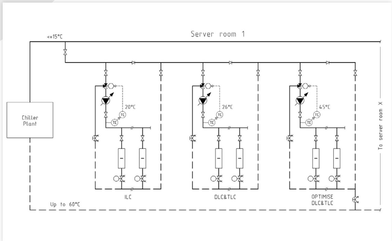
Image 11 Chiller based Temperature Chaining by Tebodin Bilfinger
