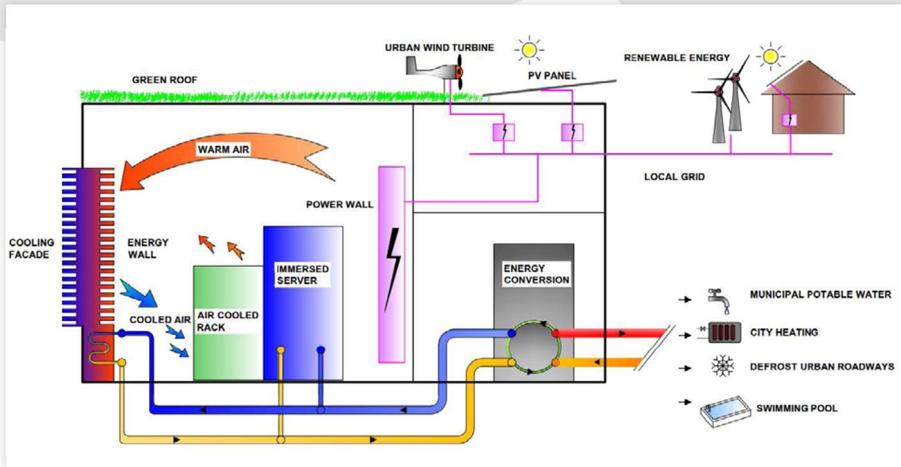
Image 14 Concept for a purpose built micro edge datacentre by Tebodin Bilfinger
