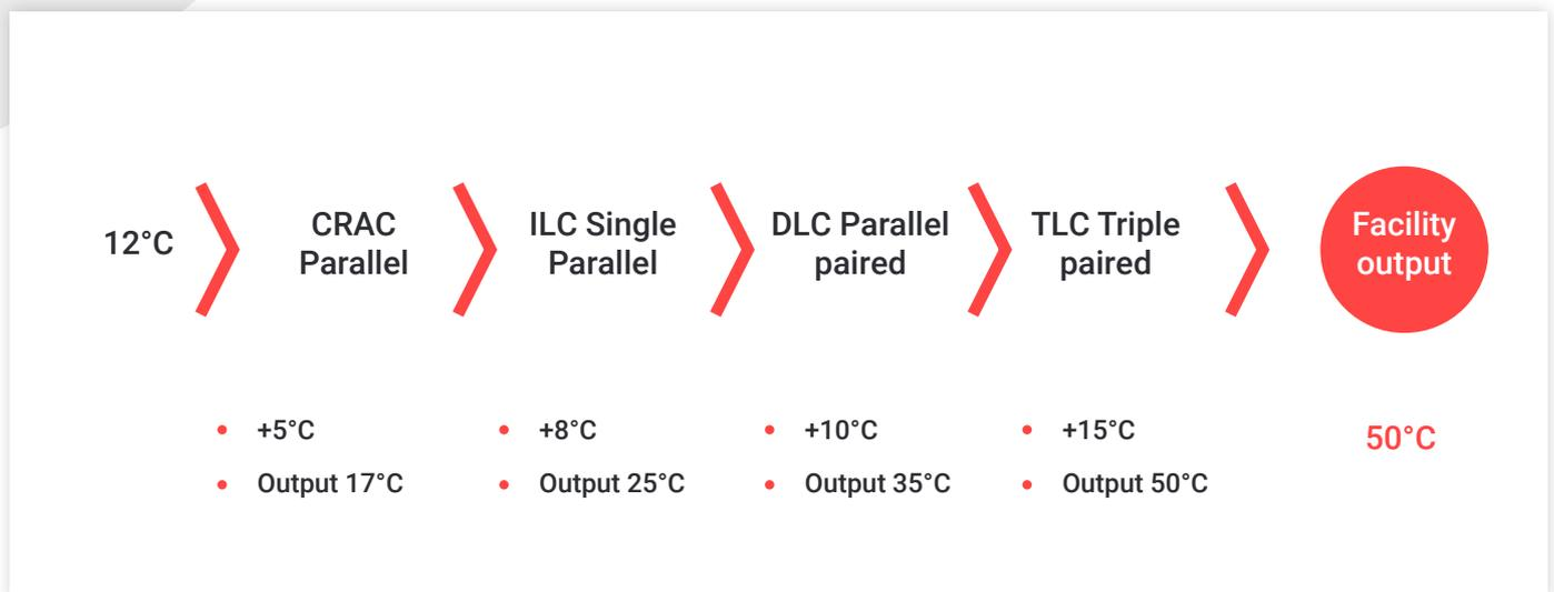
Image 6 Temperature chaining principle
